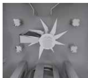
Triturador con velocidad variable / removible Speed variation in flake crusher / removable
