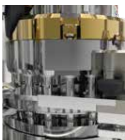
Cabezal intercambiable Interchangeable turret head
